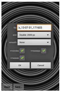
The important thing to note is that you can alter the size and quality of the saved image. Picture sizes vary from 100 pixels up to 1000/2000/4000, (the upper limit depending on the amount of internal memory in the Android device). In SourcesLite the image is restricted to screen size or 750 pixels, whichever is smaller.
